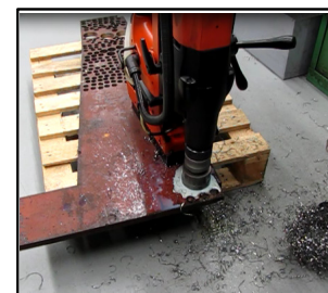
Core drilling in Hardox 400 with KBM 80 auto
